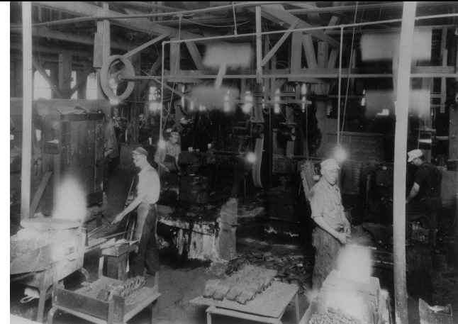
Spiller Axe Company, another of the many tool producers in Oakland. Note the axe heads in the bottom center of the picture. This section of the factory forged the steel heads.
